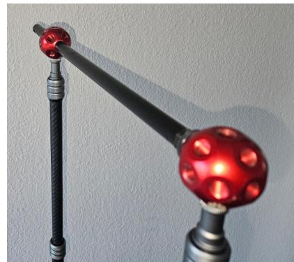
Now we screwed in two 25 cm pipes on the sides of the front red ball.
