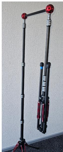
Now we have screwed on stand into one of the red balls and are about to screw in the other. Make sure, you have the stands on different levels and folded, otherwise you won't be able to screw in the stand.
