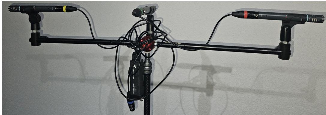
This is the complete setup of the OCT microphone system.
