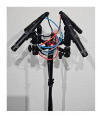
We always fasten the cable to the stand, so the full weight of the cable is not pulling the microphones down.
