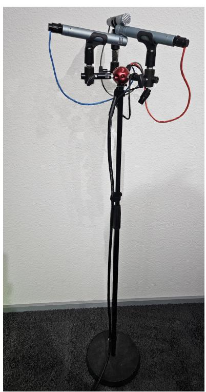
Here, the microphones are already wired up and the multicore is also secured to the microphone stand with additional cable ties.
