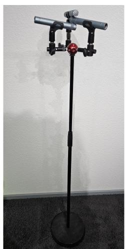
All microphones are in a different level, but the diaphragms are aligned to the Y-axes, just imagine the microphone stand is sending out a laser beam to the ceiling and you have to align all diaphragms to it.
