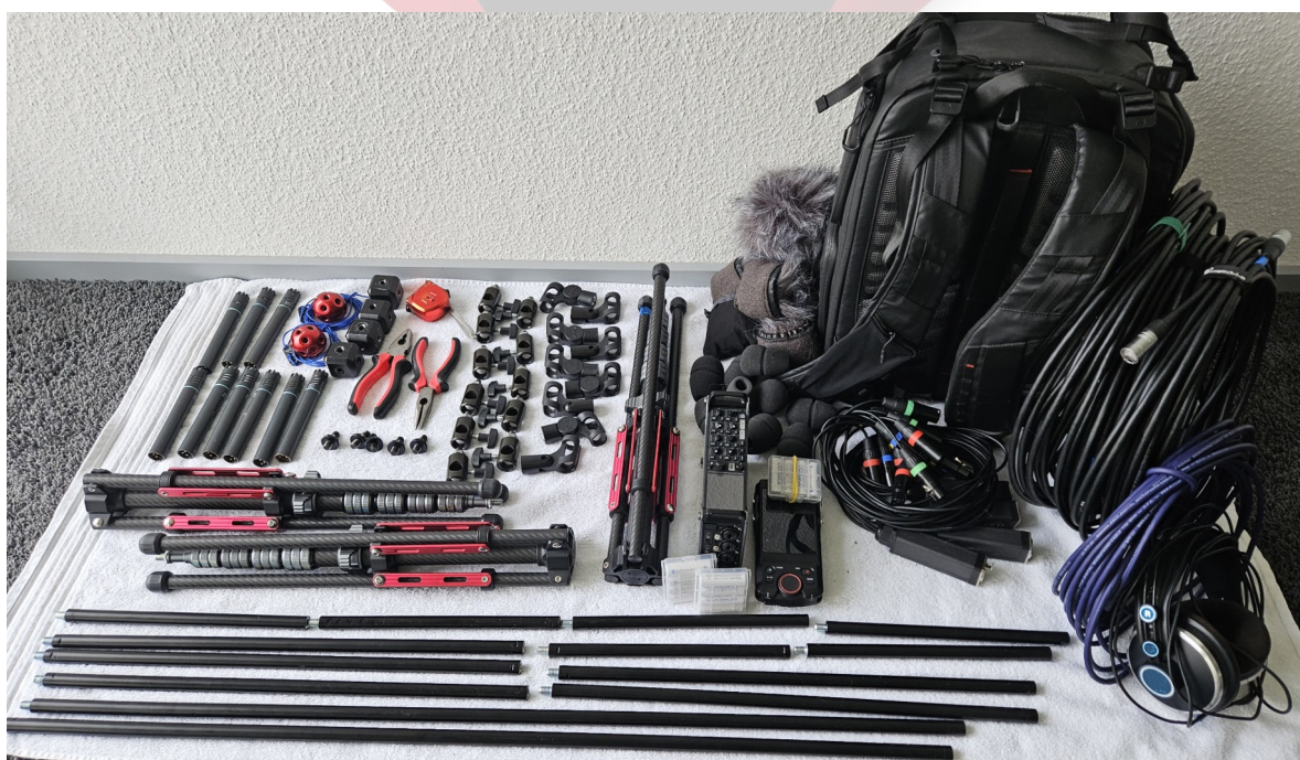
Meanwhile we exchanged the two 100 cm long pipes by four 50 cm long pipes. It's more convenient to carry!
